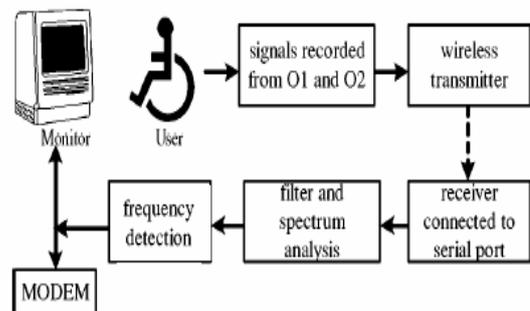
Block diagram of the SSVEP-based BCI system for expressing the user's thought
