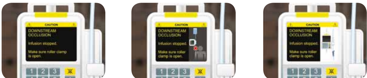
Figure 1. Alarm System Displays
